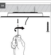
**04** Lead the connection cable through the cable membrane, fix the mounting plate with suitable mounting material, check the tight fit of the mounting plate.
