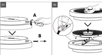
**01** Remove the locking screw on the side to be able to remove the light head.
