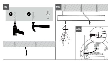
**03** Drill the holes and use the dowels for secure mounting (see also mounting instructions). **Pay attention to deeper installations when drilling!**
