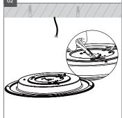
**01** Turn the mounting plate (**A**) on the back of the luminaire clockwise to open it. To facilitate mounting, release the two safety rope (**B**) from the luminaire.
