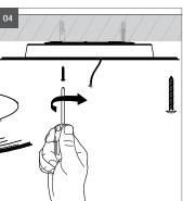
**04** Lead the connection cable through the cable membrane, fix the mounting plate with suitable mounting material, check the tight fit of the mounting plate.
