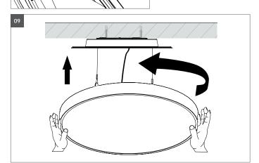
**09** To close the luminaire, place the luminaire in the correct position with the bolts in the guide openings on the mounting plate. Then turn the luminaire counterclockwise with a powerful jolt into the fixed position. Check that the luminaire is firmly seated in the mounting plate!
