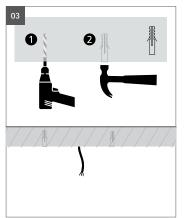
**03** Drill the holes and use the dowels for secure mounting (see also mounting instructions).
