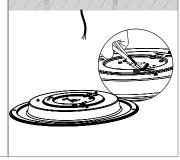
**01** Turn the mounting plate (**A**) on the back of the luminaire clockwise to open it. To facilitate mounting, release the two safety rope (**B**) from the luminaire.
