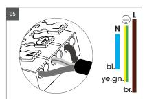
**05** Connect the cable terminals according to VDE 0100 regulations. See terminal assignment.
