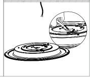
**01** Turn the mounting plate (**A**) on the back of the luminaire clockwise to open it. To facilitate mounting, release the two safety rope (**B**) from the luminaire.
