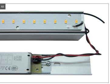
For mounting please remove black and red wire. To remove it please press on top of cable gland of each wire and pull on each carefully.
