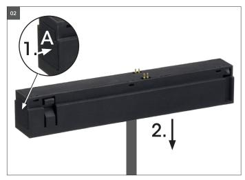
**Image 02:** To remove the LED track spotlight, press the head button **(A)** located on the base. The fastening is inactive and the LED light can easily be removed.
