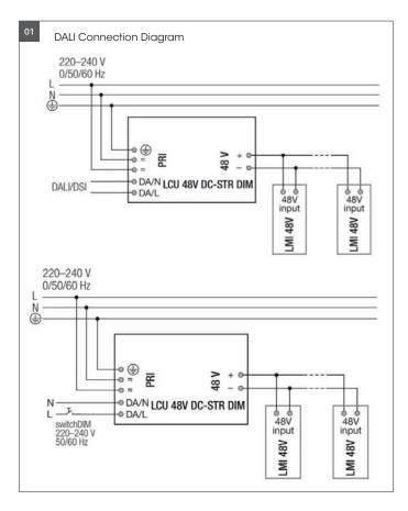
Luminaires with integrated DALI to DC Powerline communication (PLC) can only be operated with the PEP track and the compatible DC string constant voltage LED driver (art. no.: TRL-LCU75W48VDD) or TRL-LCU150W48VDD).
