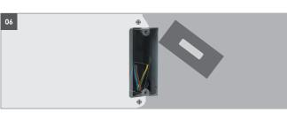
06 Apply putty to the installation housing and fastening screws. The housing must not be contaminated with putty! Then grind flat.
