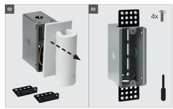
02 Remove the luminaire from the installation housing.03 Fasten mountings at the top and bottom to the installation housing with 2 threaded screws each.
