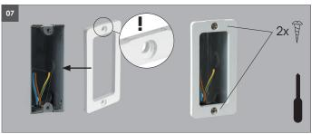
**07** Place the mounting frame in the correct position (**elevation must be at the top**) and mount it with 2 screws (included in the scope of delivery).
