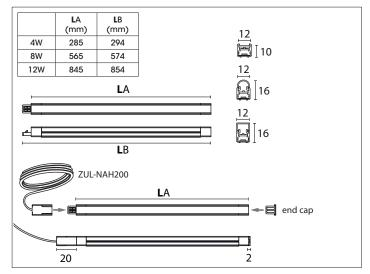
The performance of 55W when connecting light bars to each other may not be exceeded. Use new lines (power supplies) for additional lights.
