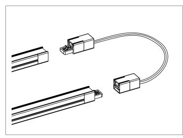
Remove the connection cover. Only use the flexible connections with each other that are intended for the original connection cable.
