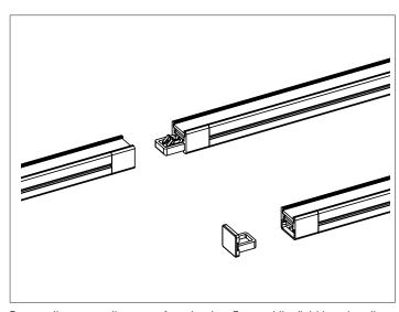
Remove the connection cover for extension. Connect the light bars together using the plug module. Check the plug contacts for fixed connection.
