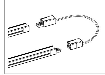
Remove the connection cover. Only use the flexible connections with each other that are intended for the original connection cable. Check the plug contacts for fixed connection.
