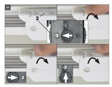
**04** Set phase with side phase selection dial **(2)** for commissioning the luminaire with the contact selection switch 1/2/3.
