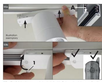
**Attention!** Adapter can only be installed in 3phase track in one direction. Locking mechanism must be placed on track side like marked with **A**.
