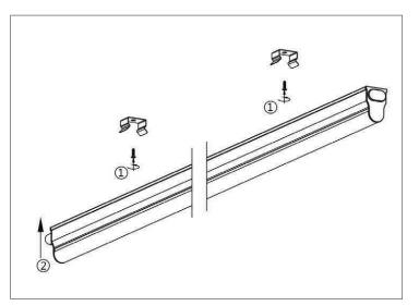
For the installation use the enclosed mounting brackets.
