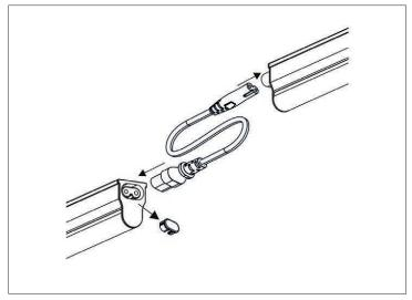
For flexible connections remove the end cap. Only the original connecting cables may be used.
