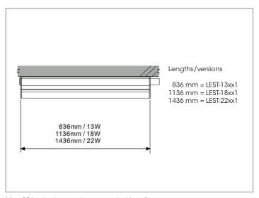
Max. 10 luminaires can be connected together.
