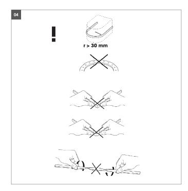
**04.** Minimum radius of bending 30 mm. **Do not bend**, bending will damaae the conductors.
