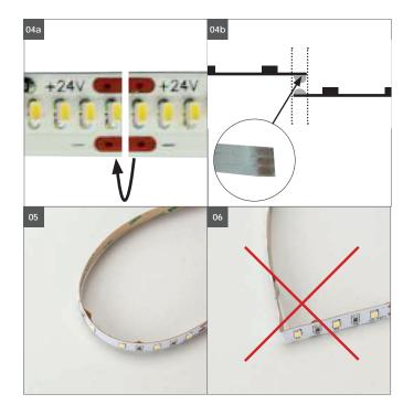
**04a.** Segments can be connected by soldering of abridge. Solder up the upper soldering point (pict. 04b) with the lower point. Soldering points become visible as soon as protection foil is taken off. Don't take off the foil completely as not to lose the adhesive power of FLEXY. Attention! Maximum 5m of Flex strip can be installed with one feeder. For more, additional feeding is required.
