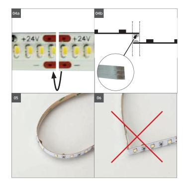
**04a.** Segments can be connected by soldering of abridge. Solder up the upper soldering point (pict. 04b) with the lower point. Soldering points become visible as soon as protection foil is taken off. Don't take off the foil completely as not to lose the adhesive power of FLEXY. Attention! Maximum 5m of Flex strip can be installed with one feeder. For more, additional feeding is required.
