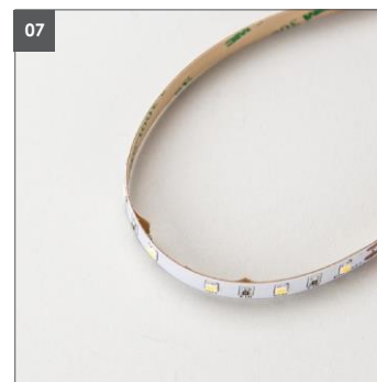
07. Minimum radius of bending 3 cm.
