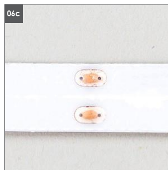
06a. Segments can be connected by soldering of a bridge. Solder up the upper soldering point (pict. 06b) with the lower point (pict. 06c). Soldering points become visible as soon as protection foil is taken off. Don't take off the foil completely as not to lose the adhesive power of FLEXY. Attention! Maximum 5m of Flex strip can be installed with one feeder. For more, additional feeding is required. Attention! When mounting on an electrical conductive base, an additional, overlapping insulation (adhesive foil) is required.
