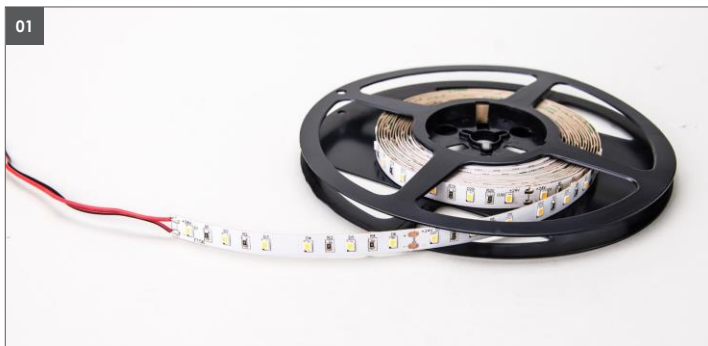
01. Only install on a suitable base (e.g. aluminium) to ensure sufficient heat transfer to the environment. Attention: When mounting on an electrical conductive base, an additional, overlapping insulation (adhesive foil) is required.
