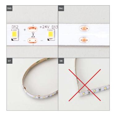
Solder up the upper soldering point (**pict. 06b**) with the lower point (**pict. 06c**). Soldering points become visible as soon as protection foil is taken off. Don't take off the foil completely as not to lose the adhesive power of FLEXY. Attention! Maximum 5m of Flex strip can be installed with one feeder. For more, additional feeding is required.
