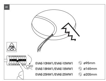
Switch off before installation. Switch on only after complete installation and examination of the circuit. Professional electrician for installation and maintenance only. Turn Off power supply before starting any installation. Read instructions & check you have all the tools & accessories to complete the installation correctly. Open a hole according to the cutout size of led downlight.
