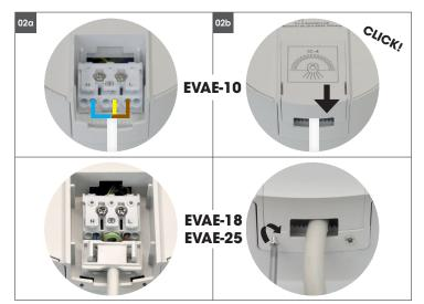
Open the driver cover. Feed the main AC wire L (4) N to the fast connection terminal block respectively. Fix the cover back.
