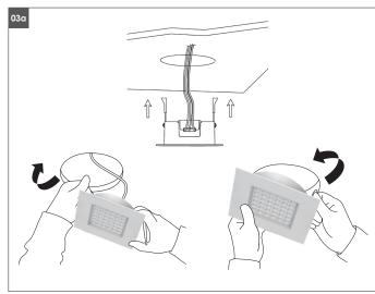
Hold back spring clips then push downlight into the hole. Make sure the downlight fixed tightly in ceiling.
