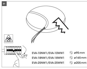
Switch off before installation. Switch on only after complete installation and examination of the circuit. Professional electrician for installation and maintenance only. Turn Off power supply before starting any installation. Read instructions & check you have all the tools & accessories to complete the installation correctly. Open a hole according to the cutout size of led downlight.
