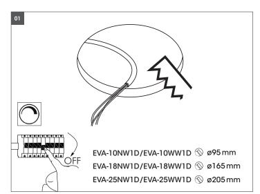
Switch off before installation. Switch on only after complete installation and examination of the circuit. Professional electrician for installation and maintenance only. Turn Off power supply before starting any installation. Read instructions & check you have all the tools & accessories to complete the installation correctly. Open a hole according to the cutout size of led downlight.
