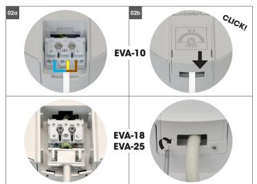
Open the driver cover. Feed the main AC wire L
