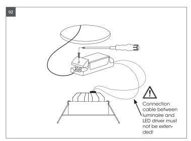
Open the driver cover. Feed the main AC wire L  $\textcircled{\oplus}$  N to the fast connection terminal block respectively. Fix the cover back.
