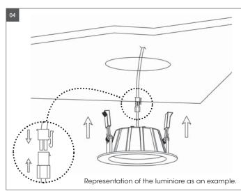
Connect the downlight with driver, hold back the spring clip then push the downlight into the hole.
