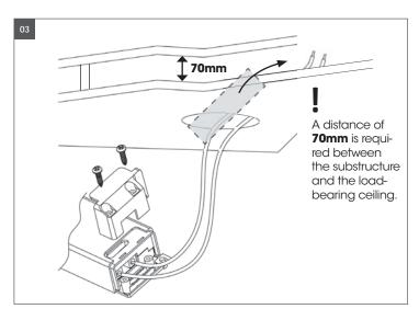
Feed the main DALI AC 230V 50Hz wire L. N. in terminal block respectively, then fix the cover back (strain relief).
