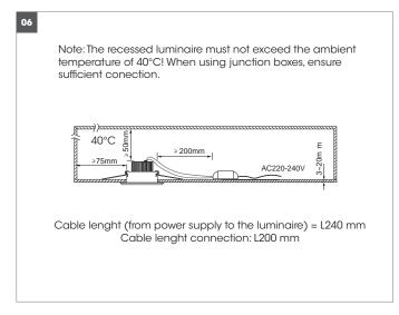
06.Please make sure to leave the distance between the lights, between the light and the provided LED power supply, and between the light and the wall. The distance from the provided LED power supply to the edge of cutting hole must be more than 200mm. Make sure the wiring and the plugs are all in correct and workable situation. After check, turn on the power.
