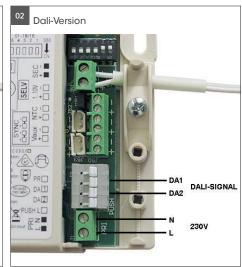
02. Connect the LED power supply to main power and connect the LED power supply with the light, see Fig. 02. Connect the wires at the power supply ohnprimary an secondary side. conductor cross-section 1,5 mm².
