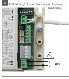
03. Connect the connection cables to the power supply, see Fig. 03. Then connect the power supply to the luminaire and connect the power supply unit to the power supply max., conductor cross section 1.5mm<sup>2</sup>.
