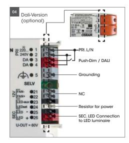
04. Connect the LED power supply to main power and connect the LED power supply with the light, see Fig. 02a. Connect the wires at the power supply ohnprimary an secondary side. conductor cross-section 1,5 mm<sup>2</sup>
