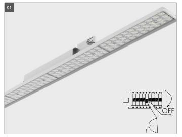
**01** Switch off before installation. Switch on only after complete installation and examination of the circuit. Professional electrician for installation and maintenance only. Turn Off power supply before starting any installation. Read instructions & check you have all the tools and accessories to complete the installation correctly.
