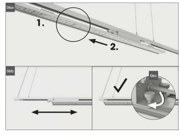
06a Several luminaires can be placed flush in succession.06b Set the end position of the luminaire.06c Fix with locking screws.
