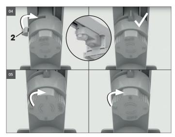
**04** Lock the retaining latches **2** and check for tight fit of the light in the track. **05** Use the contact selector switch 1/2/3 to put the luminaire into operation.
