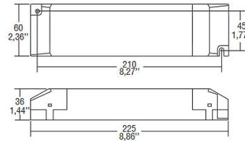
Electronic Power supply for LED, 50W 24V, SELV
